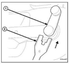
Using trim stick C-4755 or equivalent, separate the inside handle bezel cap (2) from the bezel (1).
